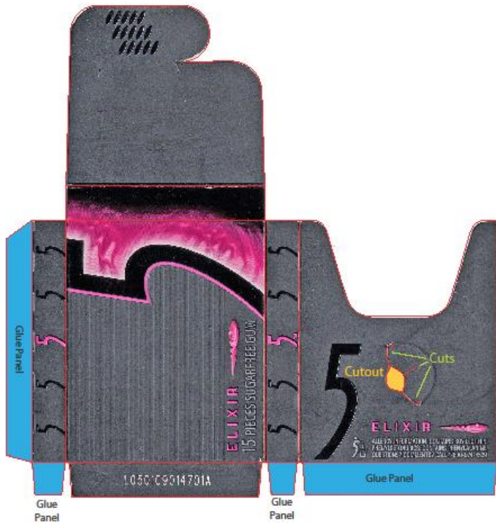
Dieline by Claytowne.com Deconstruction of Wrigley's 5 Gum Box
